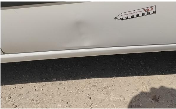
3: Wing nsf Scratched UpTo 25mm Thru Paint
