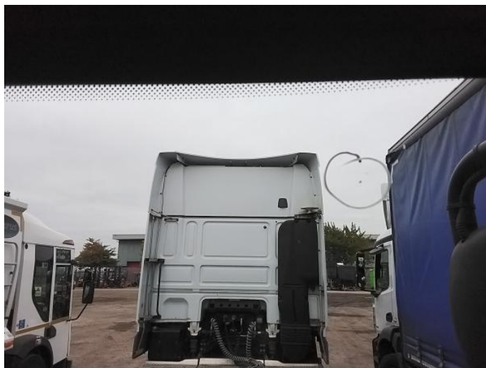
2: Screen Front Chipped UpTo 10mm
