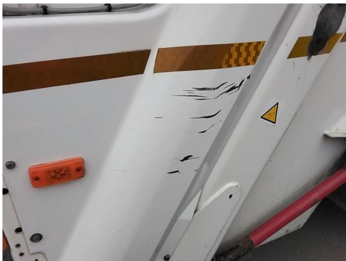
1: Qtr Panel Moulding os Scratched (Painted) Over 25mm Thru Paint
