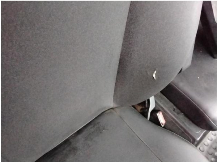
3: Seat Back Cover osf Torn Over 3mm
